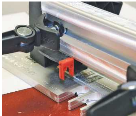
▲ This small red peg sets the correct offset for comb joints
